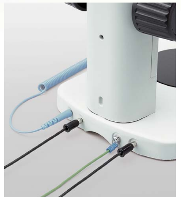
Ground wire connection (back side)
