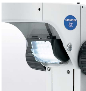
Flexible angle of LED light source
